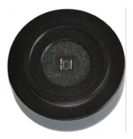
To attach the Camare to the guider telecsope there is a 4-5mm thick T2 inside screw. Any T2? 1.25" adapter can be used for 1.25" (31.7mm) focusers. There is a 1.25" filter thread inside the T2 panel to attach some filter or "dust preventor".
