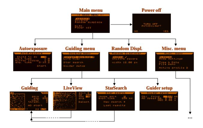
To navigate in the menu use SET and ESC buttons. SET is to enter a subscreen while ESC is to exit the current one. The previous screens and their selected items are stored in a stack, by going back to them will hold the previous selection. By entering a new one will have the default item selected on it.
