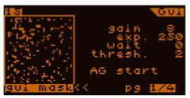
On the Guiding screen there is always the guiding star (or other) monitored in the window on the left. This is a 48x48 pixel window in a frame.
